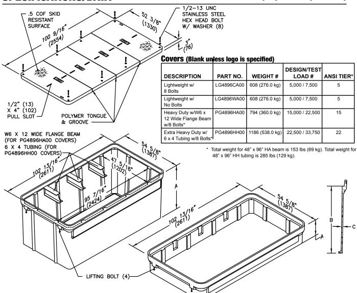
**Boxes** (Stackable with self-aligning, replaceable EZ-Nut)
